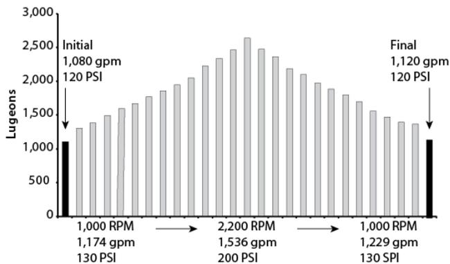
**Figure 4** - Lugeon profile for 230-ft zone observed under the revised injection mode. Symmetry about the point of maximum pressure and flow is characteristic of hydrojacking behavior and is typical of ongoing injections at CC&V.
