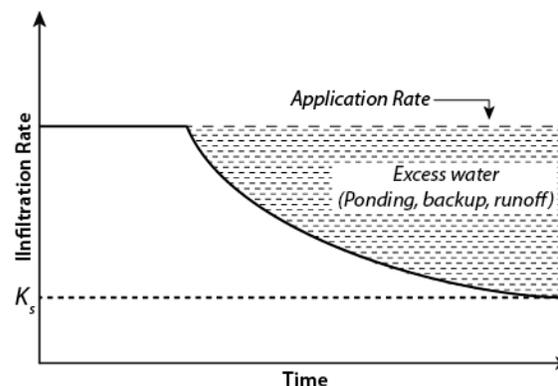
**Figure 3** - Time dependence of infiltration rate und a constant application rate higher than the saturated hydraulic conductivity of the matrix. (After Hillel [19].)
