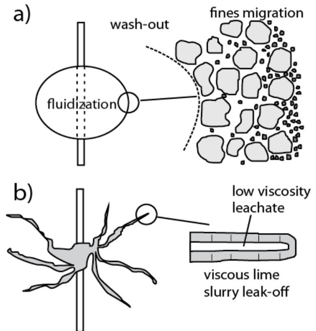
**Figure 2.** a) Schematic of injection process showing region around injection borehole with fluidization. Far from the cavity's center is an area of washout with little fines and a region of concentrated fines from migration. b) viscous fingering from lime slurry
