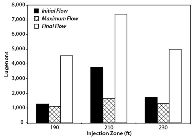
**Figure 1** - Lugeon values computed from pressure and flow rate measurements before, during, and after the injection cycle on three zones from the 2010 injection trial. Injection zones are denoted by depth from the pad surface.
